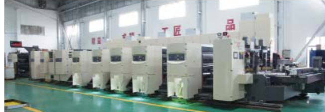
Shinko Super Alpha - Fixed structure, Servo Control Flexo Folder Gluer
